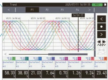
The trend graph screen displays graphs for the items per page (4 pens/page or 8 pens/page) set in the display setting. All input/output channels (Ai/Di/Oi/Do) are assigned to each pen.
