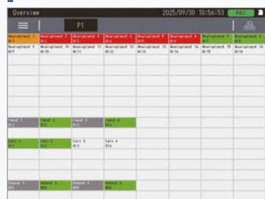
Displays the latest data for each channel. The display per screen can be selected from 16, 32, 64, or 128 points.
