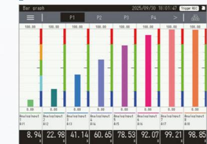
Displays the latest input/output values. Displays the channel assigned to the pen.
