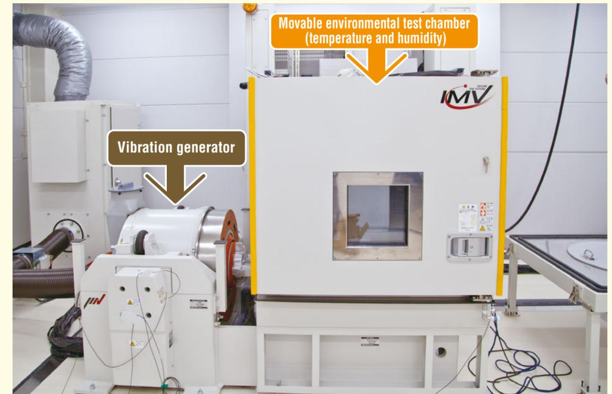
We completed the vibration testing facility at Kyoto Techno Center in June 2014. It is combined with the environmental test chamber by which the vibration test can be conducted both vertically and horizontally under the harsh environments to cover the temperature -40°C to +140°C and the humidity 20% to 90% RH.
