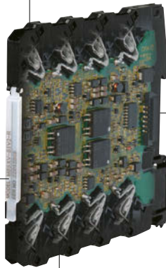
Signal conditioner (transparent view for explanation)
