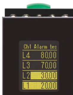
Alarm test output display
