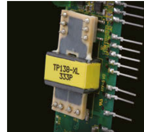
Seat transformer With the ultra-slim sheet transformer made from a printed circuit board, the M5VSH has achieved a dielectric strength of 2000 V AC without taking up much space.
