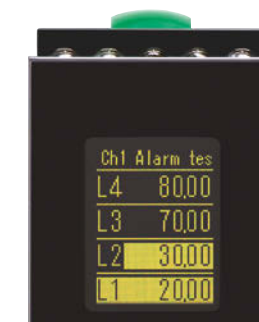
Alarm test output display
