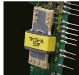
Seat transformer With the ultra-slim sheet transformer made from a printed circuit board, the M5VSH has achieved a dielectric strength of 2000 V AC without taking up much space.
