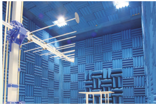
RF Anechoic Chamber
