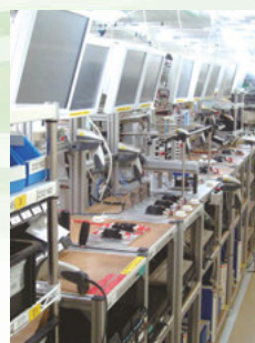
Fully computer supported test/inspection line
