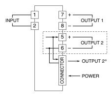
\* For 1 output channel type, OUTPUT 1 is also connected to the card-edge connector inside. Note: The section enclosed by broken line is only for 2nd output channel.
