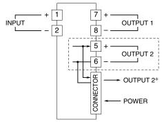
\* For 1 output channel type, OUTPUT 1 is also connected to the card-edge connector inside. Note: The section enclosed by broken line is only for 2nd output channel.
