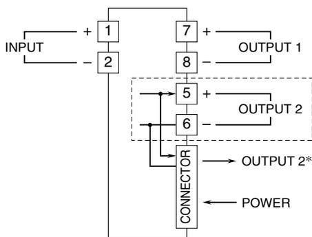
\* For 1 output channel type, OUTPUT 1 is also connected to the card-edge connector inside.
