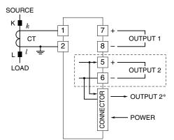
\* For 1 output channel type, OUTPUT 1 is also connected to the card-edge connector inside. Note: The section enclosed by broken line is only for 2nd output channel.
