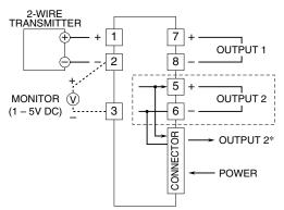
\*For 1 output channel type, OUTPUT 1 is also connected to the card-edge connector inside.
