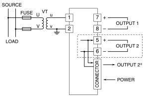
\*For 1 output channel type, OUTPUT 1 is also connected to the card-edge connector inside.
