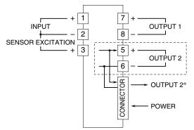
\* For 1 output channel type, OUTPUT 1 is also connected to the card-edge connector inside. Note: The section enclosed by broken line is only for 2nd output channel.
