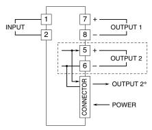
$^{st}$  For 1 output channel type, OUTPUT 1 is also connected to the card-edge connector inside. Note: The section enclosed by broken line is only for 2nd output channel.
