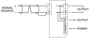
The 10VF, by its fast-response feature, is not designed to eliminate noise present in the input signal. Use a shielded twisted-pair cable for preventing noise entering through the input wiring.
