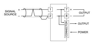
The 10VF2, by its fast-response feature, is not designed to eliminate noise present in the input signal. Use a shielded twisted-pair cable for preventing noise entering through the input wiring.
