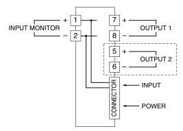
Note: The section enclosed by broken line is only for 2nd output channel.
