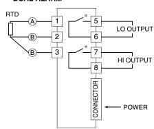
\*Relay status is determined by output codes.
