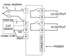
\*Relay status is determined by output codes.
