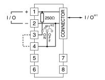
\*1. The output signal is OUTPUT 1. \*2. Jumper JP1 is factory set to "ON." Note: DO NOT connect to the terminals 5, 6, 7 and 8.
