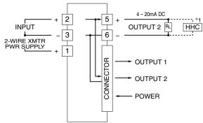
For OUTPUT 2, use either of terminals on the front or connector on the rear.
