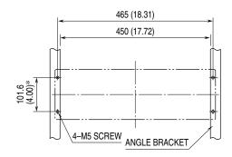
Observe an appropriate wiring space over and below. \*100 (3.94) for JIS standard
