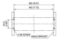
Observe an appropriate wiring space over and below.  $^{\ast100}$  (3.94) for JIS standard
