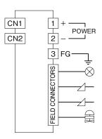
Note 1: For 18KTS and 18KJT models, directly connect input signals to input terminals of the converter and do not connect to Field Connectors. Note 2: Field Connector numbers correspond to Terminal numbers of the converters.
