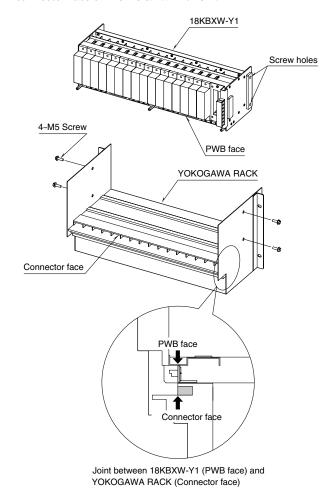
2) Fasten 18KBXW-Y1 and YOKOGAWA RACK together with screws and attach the protection cover.
