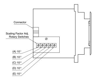
Positions for the rotary switches 10  $^{-1}$  through 10  $^{-n}$  apply respectively to each digit of the decimals and exponential as shown below.
