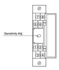
Sensitivity is adjusted with the potentiometer behind the front cover.
