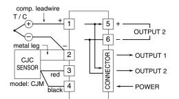
For OUTPUT 2 with current output, use either of terminals on the front or connector on the rear.
