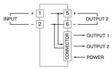
For OUTPUT 2 with current output, use either of terminals on the front or connector on the rear.
