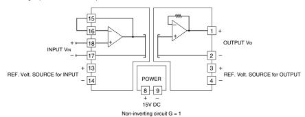
The output is proportional to the input. The gain is 1.
