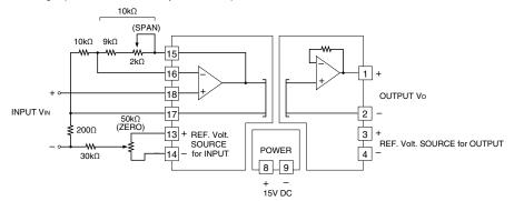
Non-inverting amplifier circuit zero/span adjustments
