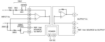
Inverting amplifier circuit zero/span adjustments
