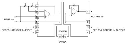
Non-inverting amplifier circuit  $G = 1 + R_1 / R_2$
