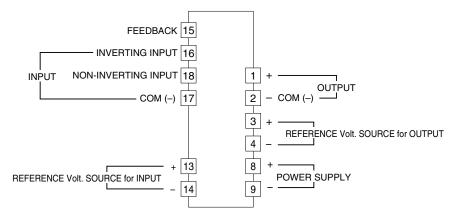
Note. The reference voltage source for input is common to the input COM (–)
