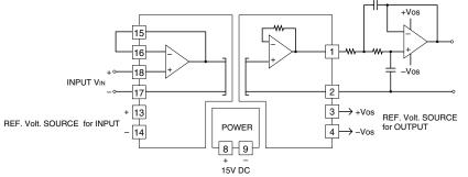
For a non-inverting amplification with external adjustments, when the combined resistance of the span adjustment and  $9k\Omega$  is  $10k\Omega$ , the gain is  $(1 + 10k\Omega / R1) \times VIN$ . With the span adjustment  $(2k\Omega)$ , the output is configurable. The zero is adjustable with a reference voltage source of  $\pm 16.5V$  DC and the attenuation of  $200\Omega$  and  $30k\Omega$ .
