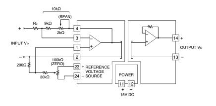
For an inverting amplification with external adjustments, when the combined resistance of the span adjustment and  $9k\Omega$  is  $10k\Omega$ , the gain is  $-(10k\Omega / R_2) \times VIN$ . With the span adjustment  $(2k\Omega)$ , the output is configurable. The zero is adjustable with a reference voltage source of  $\pm 7V$  DC and the attenuation of  $200\Omega$  and  $30k\Omega$ .
