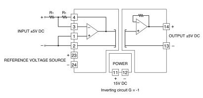
■ Inverting amplifier circuit: Basic example of G = -1 (output inverted to the input)
