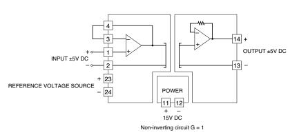
The output is proportional to the input. The gain is 1. E.g.  $\pm 5V$  DC for  $\pm 5V$  DC input.
