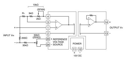
For a non-inverting amplification with external adjustments, when the combined resistance of the span adjustment and  $9k\Omega$  is  $10k\Omega$ , the gain is  $(1+10k\Omega$ /  $R_1)\times VIN.$  With the span adjustment  $(2k\Omega)$ , the output is configurable. The zero is adjustable with a reference voltage source of  $\pm 7.0V$  DC and the attenuation of  $200\Omega$  and  $30k\Omega$ .
