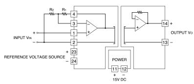
Non-inverting amplifier circuit G = 1 +  $R_1$  /  $R_2$
