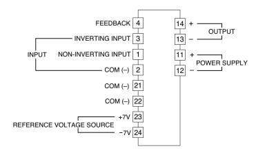
Note. The reference voltage source is common to the COM (-), terminals 2, 21 and 22.
