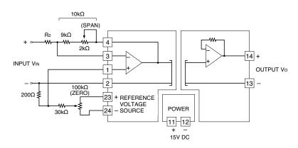
For an inverting amplification with external adjustments, when the combined resistance of the span adjustment and  $9k\Omega$  is  $10k\Omega$ , the gain is -( $10k\Omega$  /  $R_2)\times VIN$ . With the span adjustment ( $2k\Omega$ ), the output is configurable. The zero is adjustable with a reference voltage source of  $\pm 7.0V$  DC and the attenuation of  $200\Omega$  and  $30k\Omega$ .
