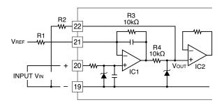
External resistors and adjusters make zero and span adjustment available.
