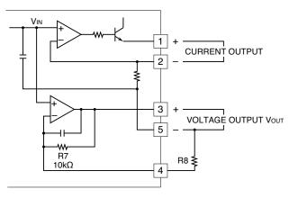
The minus terminals of current output and voltage output are not common. Do not use them at once.
