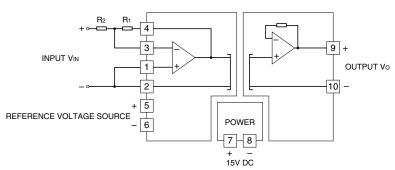
Inverting amplifier circuit G = -R1 / R2
