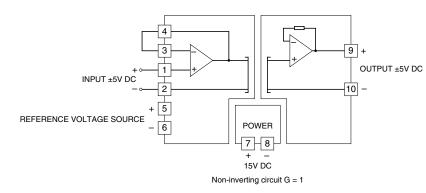
The output is proportional to the input. The gain is 1.
