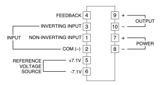
Note. The reference voltage source is common to the COM (-), terminal 2.
