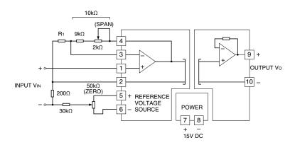
For a non-inverting amplification with external adjustments, when the combined resistance of the span adjustment and  $9k\Omega$  is  $10k\Omega,$  the gain is  $(1+10k\Omega$ /  $R_{1})\times V_{IN}.$  With the span adjustment  $(2k\Omega),$  the output is configurable. The zero is adjustable with a reference voltage source of  $\pm 7.1V$  DC and the attenuation of  $200\Omega$  and  $30k\Omega.$
