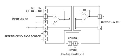
The output is inverted to the input. The gain is -1.
