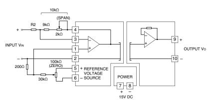
For an inverting amplification with external adjustments, when the combined resistance of the span adjustment and  $9k\Omega$  is  $10k\Omega$ , the gain is  $-(10k\Omega / R_2) \times VIN$ . With the span adjustment  $(2k\Omega)$ , the output is configurable. The zero is adjustable with a reference voltage source of  $\pm 7.1V$  DC and the attenuation of  $200\Omega$  and  $30k\Omega$ .
