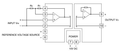
Non-inverting amplifier circuit G = 1 + R<sub>1</sub> / R<sub>2</sub>
