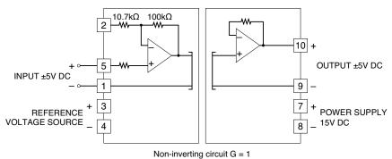
The output is proportional to the input. The gain is 1.
