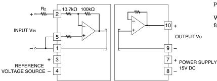
Inverting amplifier circuit G =  $-100k\Omega$  / (10.7k $\Omega$  + R<sub>2</sub>)
