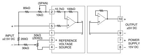
Non-inverting amplifier circuit zero/span adjustments (input ±2.5V, output ±5V)
