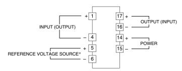
\*To be used in the printed wiring board on which the unit is mounted. Note. The reference voltage source is common to the terminal 4 (-).
