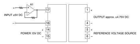
Note: The amplifier A1 requires a power source independent from the Reference Voltage Source.
