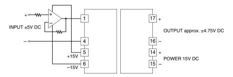
■ Non-inverting amplifier circuit: G = 0.95 (Isolation: Output to input or power)
