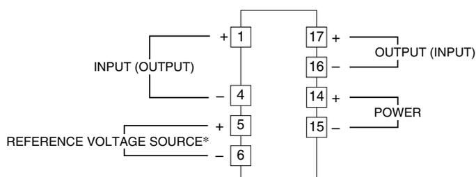
\*To be used in the printed wiring board on which the unit is mounted.
