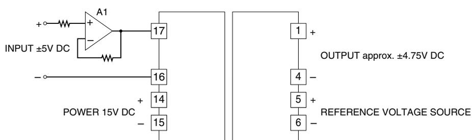
Note: The amplifier A1 requires a power source independent from the Reference Voltage Source.
