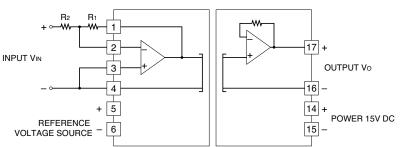
Inverting amplifier circuit G = -R1 / R2
