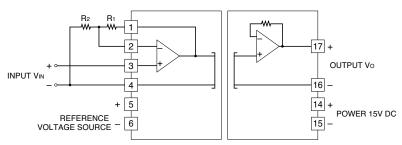
Non-inverting amplifier circuit G = 1 + R<sub>1</sub> / R<sub>2</sub>
