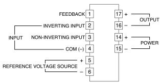
Note. The reference voltage source is common to the COM (–), terminal 4.
