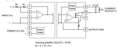
For an inverting amplification the output is following.
