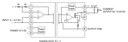
The output is inverted to the input. E.g. 20-0 mA for -5-0V input
