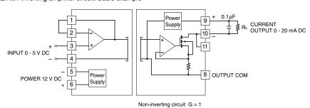
The output is proportional to the input. E.g. 0-20 mA for 0-5V DC input
