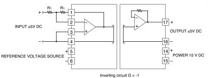
The output is inverted to the input. The gain is -1.
