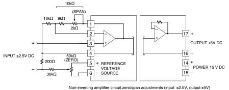
For a non-inverting amplification with external adjustments, when the combined resistance of the span adjustment and  $9k\Omega$  is  $10k\Omega$ , the gain is  $(1 \pm 10k\Omega / R_1) \times VIN$ . With the span adjustment  $(2k\Omega)$ , the output is configurable. The zero is adjustable with a reference voltage source of  $\pm 14V$  DC and the attenuation of  $200\Omega$  and  $30k\Omega$ .
