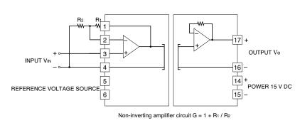
For a non-inverting amplification the output is following.  $Vo = (1 + R1 \, / \, R2) \times V{\rm IN}$
