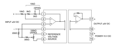
Inverting amplifier circuit zero/span adjustments (input ±5V, output ±5V)
