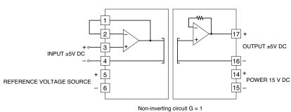
The output is proportional to the input. The gain is 1. E.g.  $\pm 5V$  DC for  $\pm 5V$  DC input.
