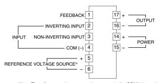
Note. The reference voltage source is common to the COM (–), terminal 4.  $^*\text{To}$  be used in the printing wiring board on which the unit is mounted.
