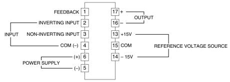
Note. The reference voltage source is common to the output (–).
