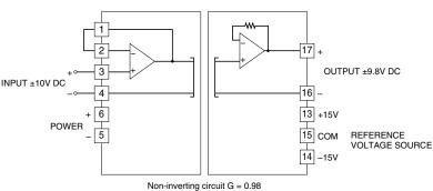
The output is proportional to the input. The gain is 0.98. E.g. ±9.8V DC for ±10V DC input.
