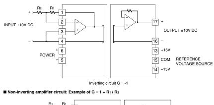
For a non-inverting amplification the output is following.  $VO = (1 + R_1 / R_2) \times VIN$ When  $R_1 = 10k\Omega$ ,  $R_2 = 10k\Omega$ , then the output is following. The gain is 2.
