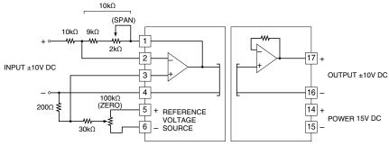
Inverting amplifier circuit zero/span adjustments (input ±10V, output ±10V)
