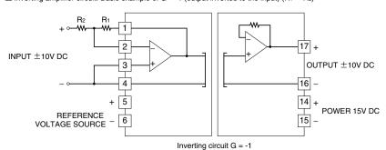
The output is inverted to the input. The gain is -1.
