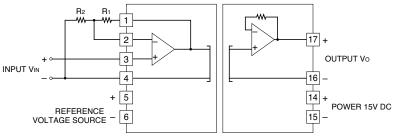
Non-inverting amplifier circuit G = 1 + R<sub>1</sub> / R<sub>2</sub>
