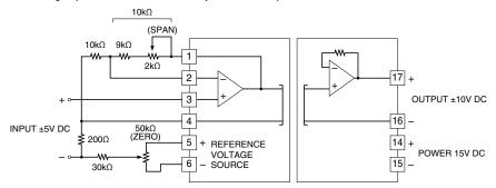
Non-inverting amplifier circuit zero/span adjustments (input ±5V, output ±10V)
