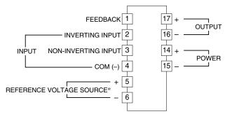
Note. The reference voltage source is common to the COM (-), terminal 4. \*To be used in the printing wiring board on which the unit is mounted.
