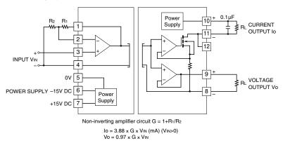
For a non-inverting amplification the output is following.
