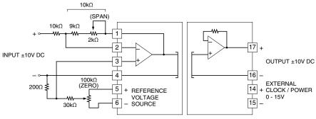
Inverting amplifier circuit zero/span adjustments (input ±10V, output ±10V)
