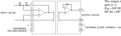
The output is inverted to the input. The gain is -1.
