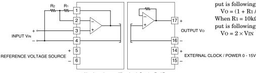
For a non-inverting amplification the output is following.
