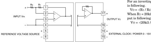
Inverting amplifier circuit G = -R1 / R2
