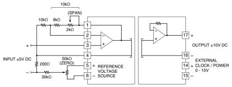
Non-inverting amplifier circuit zero/span adjustments (input ±5V, output ±10V)
