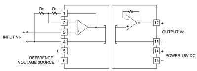
Non-inverting amplifier circuit  $G = 1 + R_1 / R_2$
