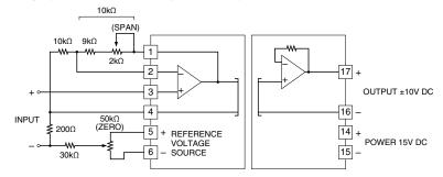
For a non-inverting amplification with external adjustments, when the combined resistance of the span adjustment and  $9k\Omega$  is  $10k\Omega,$  the gain is  $(1+10k\Omega$  /  $R_1)\times VIN. With the span adjustment <math display="inline">(2k\Omega),$  the output is configurable. The zero is adjustable with a reference voltage source of  $\pm 15V$  DC and the attenuation of  $200\Omega$  and  $30k\Omega.$
