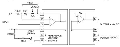
For an inverting amplification with external adjustments, when the combined resistance of the span adjustment and  $9k\Omega$  is  $10k\Omega$ , the gain is -(10k $\Omega$  /  $R_2) \times$  VIN. With the span adjustment (2k $\Omega$ ), the output is configurable. The zero is adjustable with a reference voltage source of  $\pm 15V$  DC and the attenuation of  $200\Omega$  and  $30k\Omega$ .
