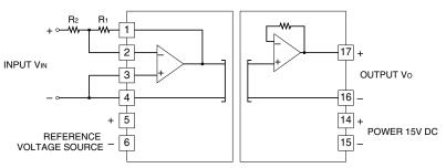
Inverting amplifier circuit G = -R<sub>1</sub> /  $R_2$
