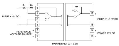
The output is inverted to the input. The gain is -0.98.
