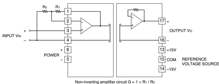
For a non-inverting amplification the output is as following.
