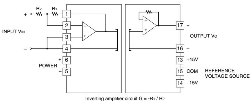
For an inverting amplification the output is as following.
