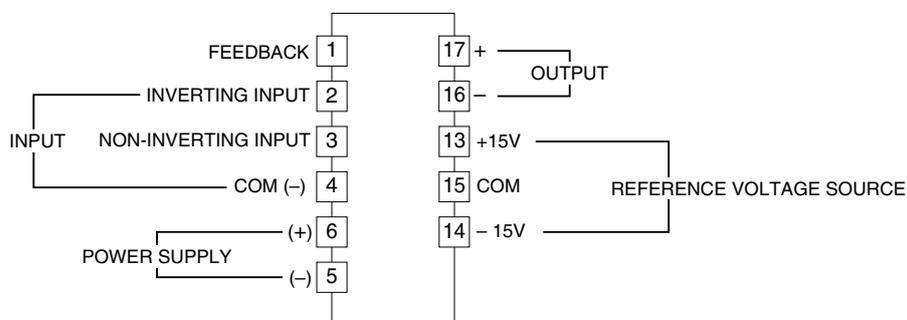
Note. The reference voltage source is common to the COM (-), terminal 4.
