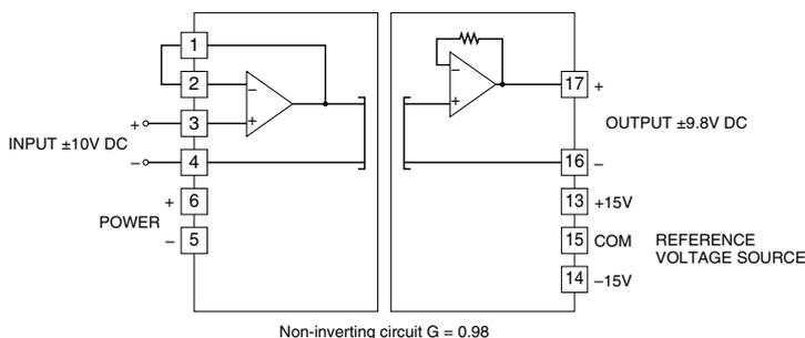
The output is proportional to the input. The gain is 0.98.
