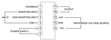
Note. The reference voltage source is common to the COM (–), terminal 4.
