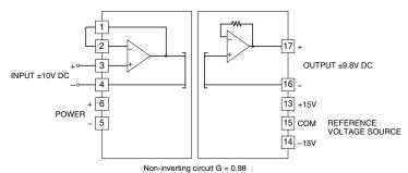
The output is proportional to the input. The gain is 0.98. E.g.  $\pm 9.8V$  DC for  $\pm 10V$  DC input.
