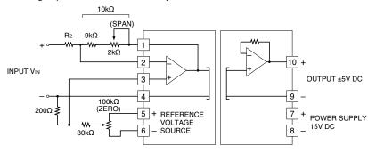
For an inverting amplification with external adjustments, when the combined resistance of the span adjustment and  $9k\Omega$  is  $10k\Omega$ , the gain is  $-(10k\Omega / R_2) \times VIN$ . With the span adjustment  $(2k\Omega)$ , the output is configurable. The zero is adjustable with a reference voltage source of  $\pm 7.5V$  DC and the attenuation of  $200\Omega$  and  $30k\Omega$ .
