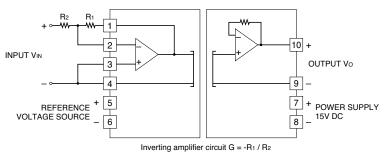
For an inverting amplification the output is following.
