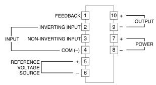
Note. The reference voltage source is common to the COM (–), terminal 4.
