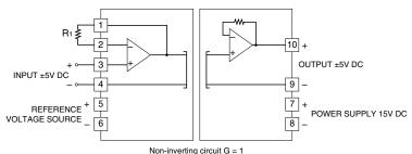
The output is proportional to the input. The gain is 1.
