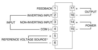
Note. The reference voltage source is common to the COM (-), terminal 4. \*To be used in the printing wiring board on which the unit is mounted.
