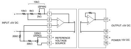
Inverting amplifier circuit zero/span adjustments (input  $\pm 5V$ , output  $\pm 5V$ )
